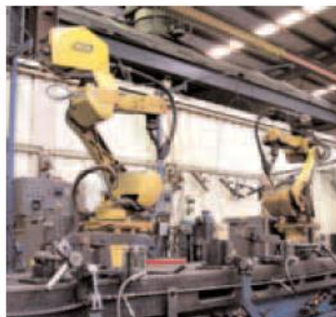
Twin Robot Cell for Molnar 4 Post Hoist Ramp Welding.
