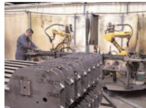
Twin Robot Cell for Molnar 4 Post Hoist Crossbeam Welding.
